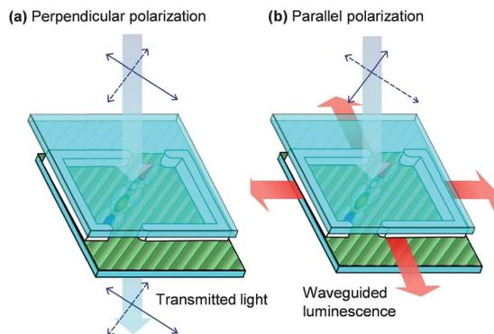
**Fig. 1** Orientation of fluorescent and dichroic dye molecules along the direction of rubbed polyamide channels by liquid crystal induced alignment. This configuration allows a luminescent solar concentrator to work as a polarizer. (a) Light with perpendicular polarization to the fluorescent dye molecules is transmitted. (b) Light with parallel polarization to the fluorescent dye molecules is captured and then reemitted and waveguided to the edges.
