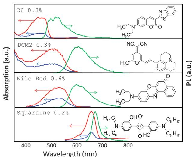
**Fig. 2** Absorption for parallel (red line) and perpendicular (blue line) polarizations and PL (green line) of four different LP-LSCs with one dye and MLC-2091 as a host material. The concentration of each dye is the same as that of the concentration of the dye in the LP-LSC with multiple dyes.
