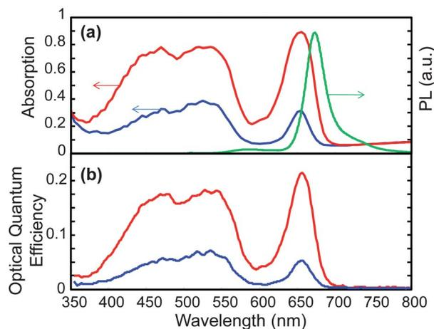
**Fig. 3** (a) Absorption for parallel (red line) and perpendicular (blue line) polarizations and PL (green line) of a device with multiple dyes and a MLC-2091 liquid crystal host (C6 0.3 wt%, DCM2 0.3 wt%, Nile Red 0.6 wt%, squaraine 0.2 wt%). (b) Optical quantum efficiency versus wavelength of the device for incident light with parallel (red line) and perpendicular (blue line) polarizations.
