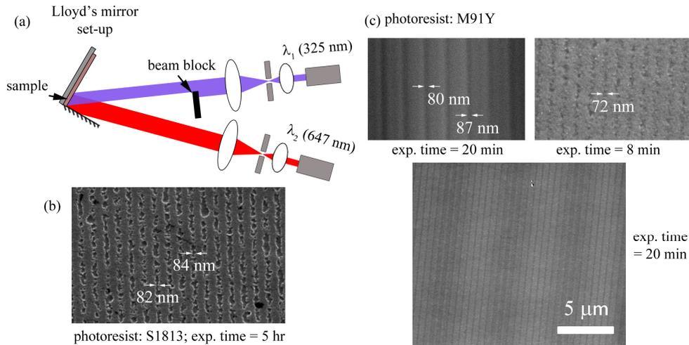
Fig. 4. (a) Modified Lloyd's mirror interferometer for proof-of-principle AMOL exposures. (b) Lines of width  $\sim 80$  nm fabricated in S1813 photoresist at an intensity ratio of 4000. (c) Lines of width  $\sim 70$ -80nm created in sensitized M91Y photoresist at an intensity ratio of 4000.
