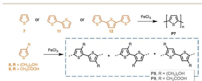
Scheme 3 Reactive vapor deposition of semiconducting polymers.
