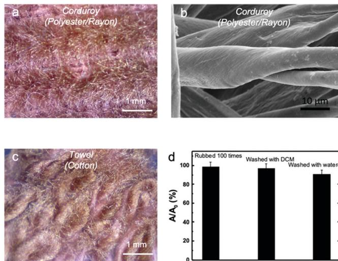
Fig. 4 (a) Optical micrograph and (b) SEM of a corduroy fabric vapor coated with **P13** in Chamber 2 (after rinsing). (c) Optical micrograph of a cotton towel vapor coated with **P13** in Chamber 2 (after rinsing). (d) Percent change in surface color of a **P13**-coated cotton towel after rubbing and solvent washing. Adapted with permission from ref. 74.
