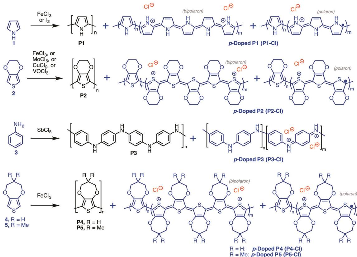
Scheme 2 Reactive vapor deposition of conducting polymers.
