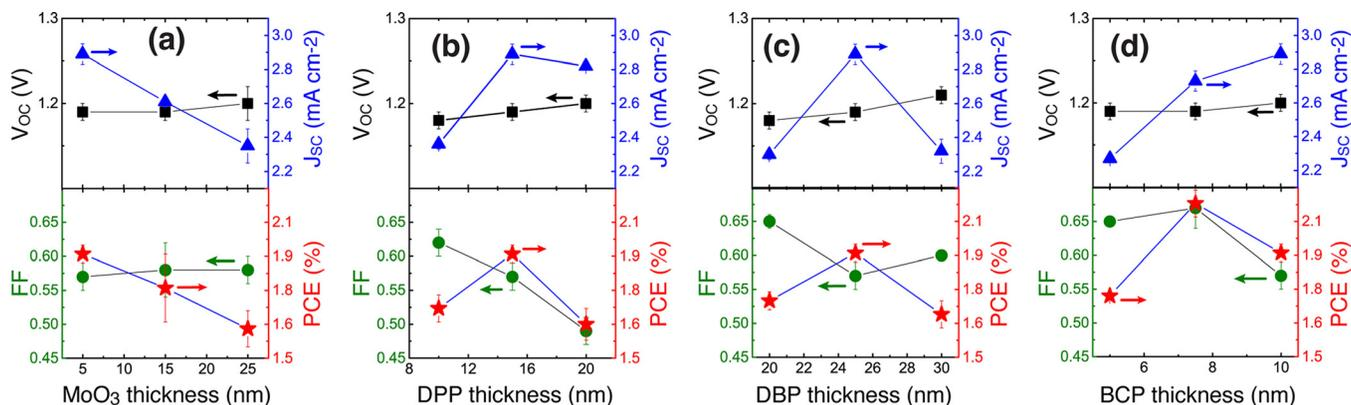
FIG. 2. Variation of  $V_{oc}$  (black squares),  $J_{sc}$  (blue triangles), FF (green dots), and PCE (red stars) for planar heterojunction devices with different MoO<sub>3</sub>, DPP, DBP, and BCP layer thicknesses. All devices were measured under 1 sun.
