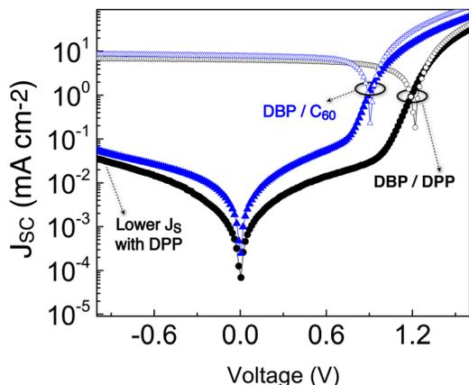
FIG. 4. Semi-log scale J-V curve in the dark (filled) and under 1 sun (open) for DPP (black circles) and C<sub>60</sub> (blue triangles) based OPVs.
