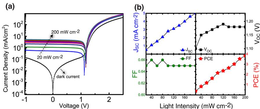
FIG. 3. Performance characteristics ( $J_{sc}$ ,  $V_{oc}$ , FF, and PCE) of the optimized DBP/DPP PHJ solar cell as a function of incident light intensity. A maximum PCE of 3.8% is achieved at 200 mW/cm<sup>2</sup>.
