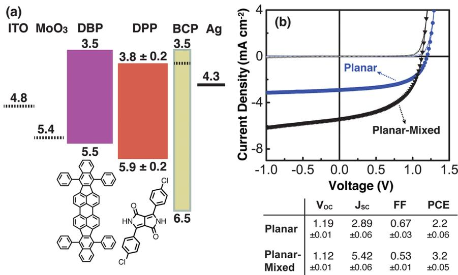
FIG. 1. (a) The energy band structure of a fullerene-free solar cell containing a DBP-DPP planar heterojunction, including the chemical structures of DBP and DPP. (b) Representative current density-voltage characteristics of both planar and planar-mixed DBP/DPP heterojunction solar cells. The current densities under light (filled symbols) were measured under 1 sun. The inset details median values of pertinent device metrics obtained over 20 devices.
