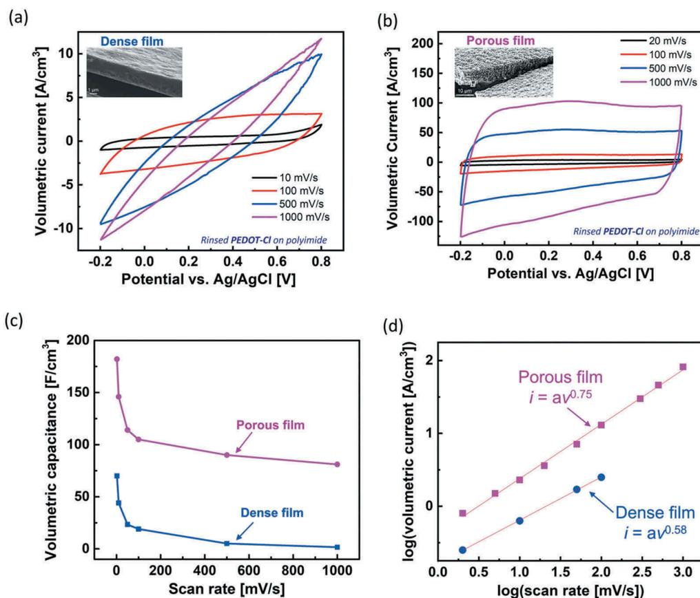
**Figure 3.** Electrochemical correlation to changes in film porosity. a,b, Three-electrode cyclic voltammetry of dense (a) and porous (b) PEDOT-Cl films (after acid rinsing). c,d Scan rate dependence of volumetric capacitance of porous and dense films. Log-log plot (d) with labelled  $i$ - $v$  relationships.
