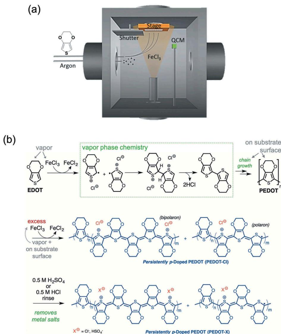
**Figure 1.** Reactive vapour deposition of persistently doped polymer films. a, Illustration of reactive vapour deposition chamber. b, Vapour phase chemistry and structure of doped conducting polymer film. Iron (III) chloride serves to both polymerise EDOT and to oxidise PEDOT (supplying a chloride counterion), forming persistently *p*-doped PEDOT-Cl. An acid rinse removes metal salts and results in counterion exchange to an ill-defined extent.
