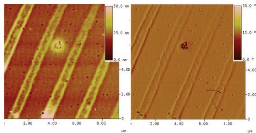
**Figure 3.** AFM height (left) and phase (right) images of a 196 nm thick film of **P1** after exposure to a parallel line interference pattern (400 nm, 2 mW, 150 fs pulses, at 60 Hz for 10 s). The circular mark near the center corresponds to a film defect.
