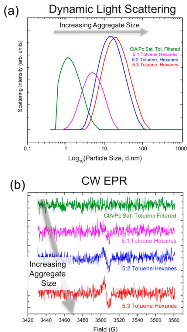
**Figure 3.** Aggregation-dependent evolution of paramagnetic EPR signal for CIAIPc. (a) Observing increasing CIAIPc aggregate size in various solvent/nonsolvent mixtures via dynamic light scattering measurements. (b) Correlated EPR spectra in various solvent/nonsolvent mixtures.
