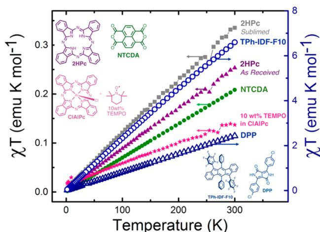
**Figure 2.** Magnetic susceptibility measurements of selected closed-shell chromophores. For clarity, the  $\chi T$  values for DPP and TPh-IDF-F10 are plotted on a separate (right) axis.
