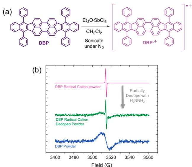
**Figure 4.** Generation (a) and dedoping (compensation) of the chemical generated DBP radical cation sample. We see in the powder EPR spectra (b) that the sharp signal from the chemically generated radical cation is distinct from the intrinsic paramagnetic state in the DBP powder.
