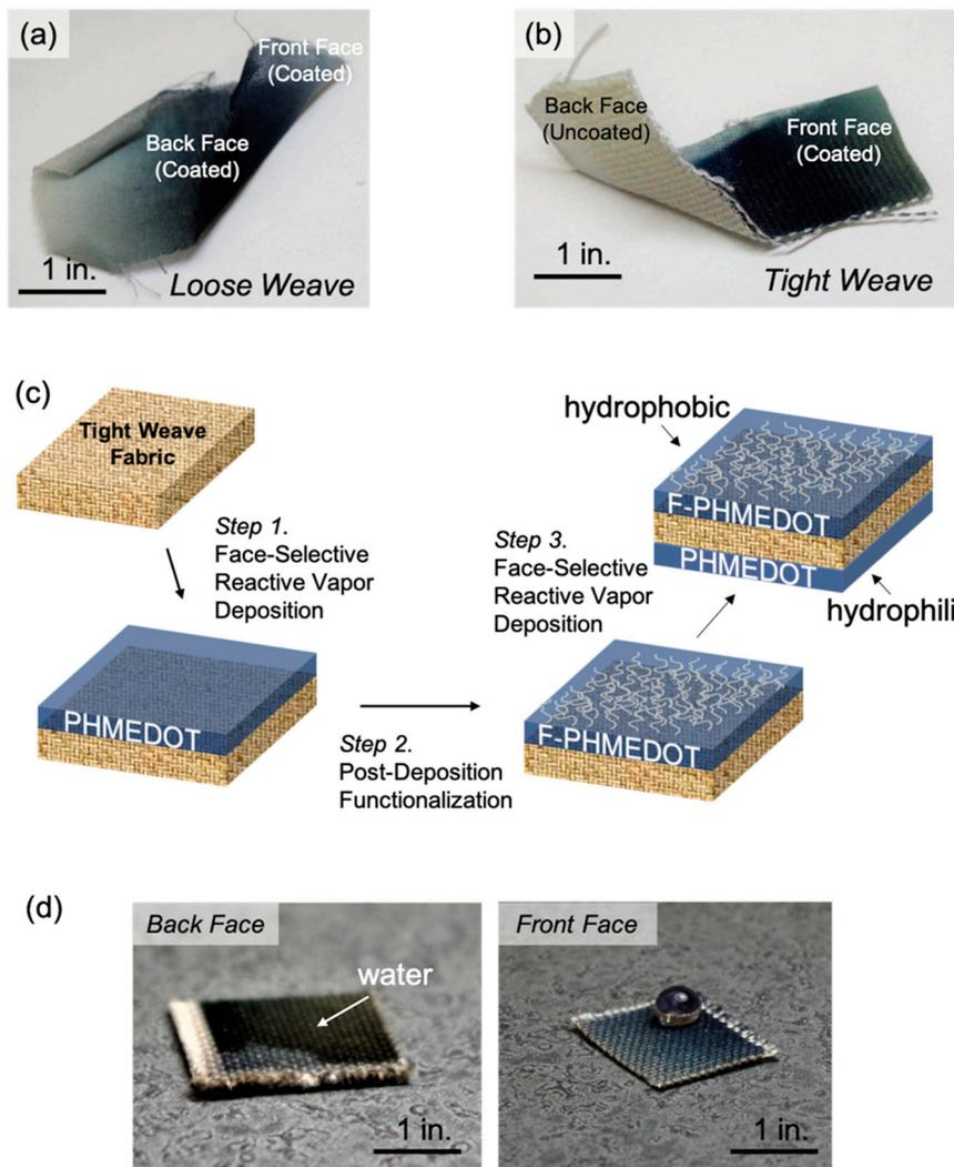
**Figure 4.** (a) Optical image of a loose weave, untreated cotton fabric vapor coated with PHMEDOT. (b) Optical image of a tight weave, untreated cotton fabric vapor coated with PHMEDOT. (c) Stepwise process for creating Janus fabrics with dissimilar wettability on each face. (d) Optical images of a water droplet on the front and back sides of the Janus fabric.
