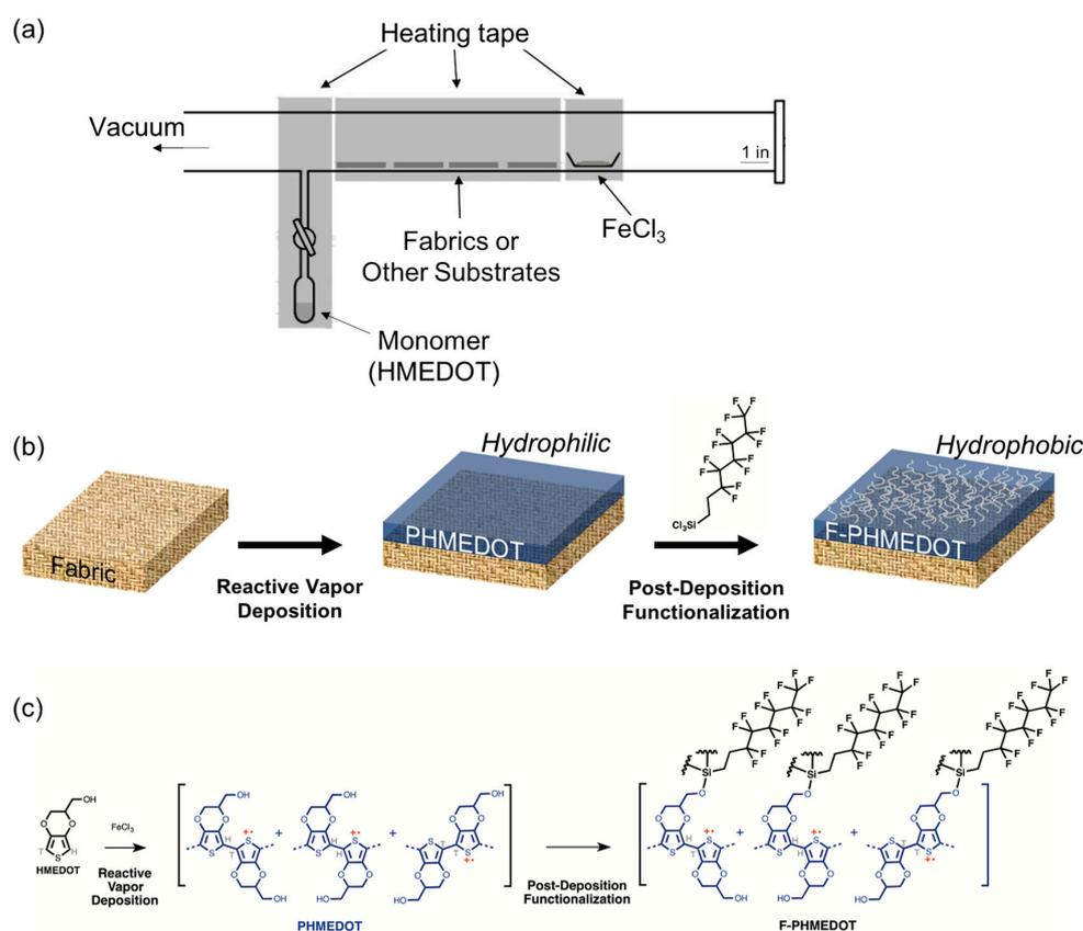
**Figure 1.** (a) Schematic of custom-built reactor used to coat untreated fabrics via reactive vapor deposition. (b) Illustration of the process to tune the wettability of off-the-shelf fabrics using reactive vapor deposition and post-deposition functionalization. (c) Chemical structures of poly(3,4-(hydroxymethyl)ethylenedioxy-thiophene) (PHMEDOT) and F-PHMEDOT polymer coatings on fabrics.
