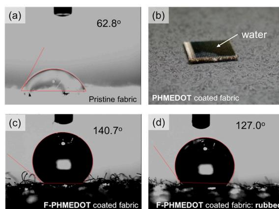
**Figure 2.** (a) Apparent water contact angle of a pristine, tight-woven, raw cotton fabric. (b) Photograph of a tight-woven, raw cotton fabric after vapor coating with PHMEDOT, showing the extreme hydrophilicity of the fabric surface. A water droplet placed on this coated fabric surface is immediately absorbed into the fabric. (c,d) Apparent water contact angles of (c) a tight-woven cotton fabric after vapor coating with F-PHMEDOT, and (d) the same vapor-coated fabric after mechanical rubbing.
