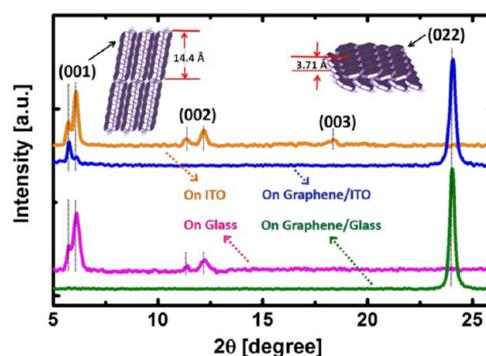
**Figure 1.** X-ray diffraction (XRD)  $\theta$ – $2\theta$  scans of pentacene films grown on bare glass, bare ITO, monolayer graphene-covered glass, and monolayer graphene-covered ITO.
