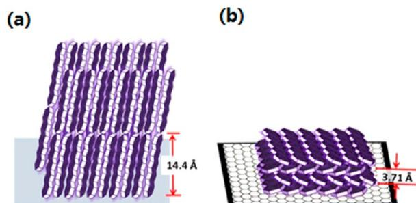
**Figure 2.** (a) Illustration of pentacene standing-up orientation on oxide. (b) Illustration of pentacene lying-down orientation on graphene.
