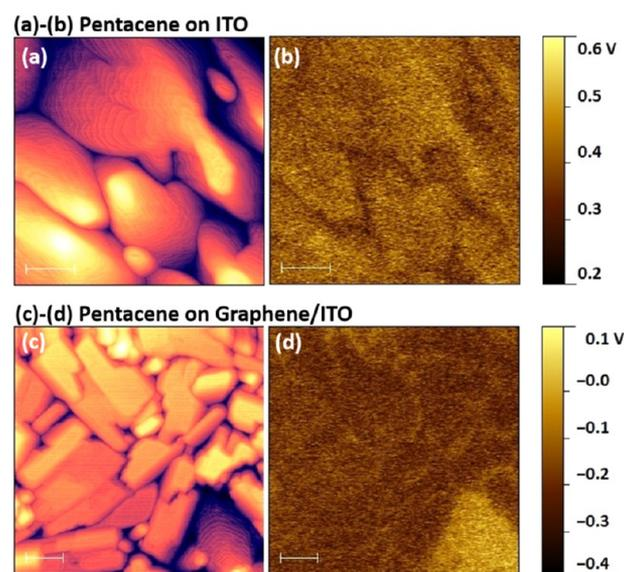
**Figure 5.** (a) Topography image of a 100 nm-thick pentacene film grown on bare ITO and (b) the corresponding CPD image measured using KPFM. (c) Topography image of a 100 nm-thick pentacene film grown on monolayer graphene-covered ITO and (d) the corresponding CPD image. Scale bar is 200 nm in all images.
