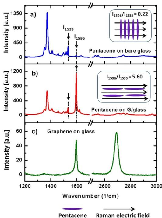
**Figure 3.** Spatially averaged Raman spectra of (a) pentacene on bare glass, (b) pentacene on monolayer graphene-covered glass, and (c) monolayer graphene on glass ( $\lambda = 532$  nm; 3.0 mW).
