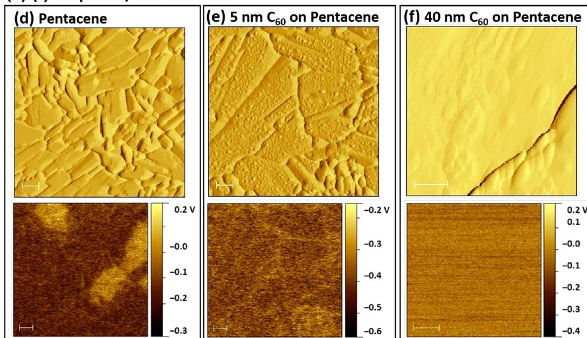
**Figure 6.** (a,d) Amplitude and corresponding CPD images measured by KPFM of 100 nm pentacene, (b,e) 5 nm  $C_{60}$  grown on pentacene, and (c,f) 40 nm  $C_{60}$  grown on pentacene; (a–c) on glass substrate, and (d–f) on graphene/glass substrate. In each box, the top image is amplitude, the bottom image is the corresponding CPD. Scale bar is 200 nm in all images.
